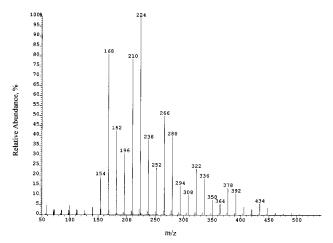
**Figure 5.** FIMS of AlCl<sub>3</sub>-catalyzed poly(isobutylene) distillate.
