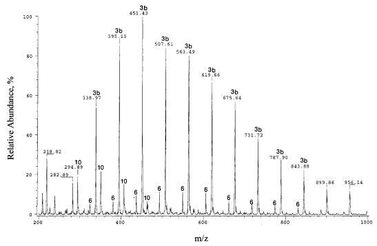
Figure 1. Negative ion ESI-MS of OLOA 15500 prepared from BF3-catalyzed poly(isobutylene).
